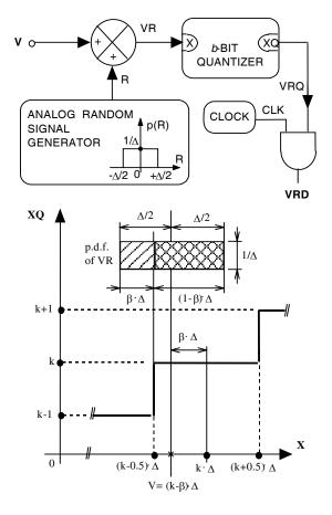
Figure 1 Analog/stochastic data converter
