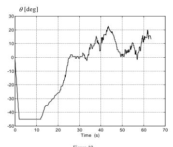
Figure 10 The FLC output  $\theta$  during docking when the input variables,  $\varphi$  and *x*, are represented by 4-bit stochastic data (from [16])
