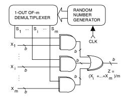
Figure 3 Arithmetic addition of *m* stochastic data streams  $X_1, X_2, ..., X_m$
