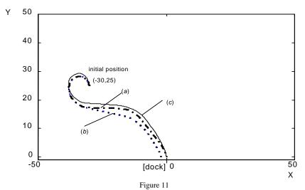
Truck trails for different FLC architectures: (a) analog ; (b) 4-bit purely digital, and (c) 4-bit stochastic data with 20-unit moving average filter (from [16])
