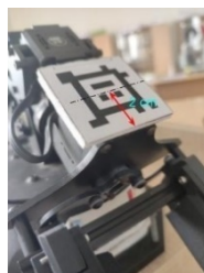
Figure 8 AprilTag's position on the robot
